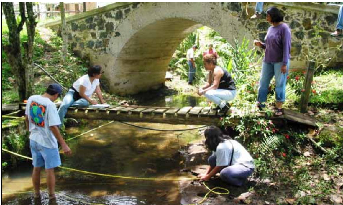
GWW-Veracruz citizen monitors being trained by Alabama Water Watch to measure stream discharge following the protocol developed earlier in the Philippines.
